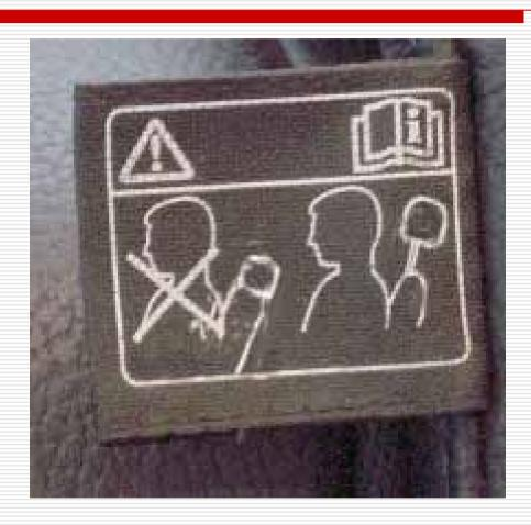
Warning label coupled with owner's manual verbiage to educate occupant as to correct head restraint positioning
