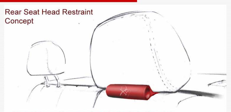
The warning tag could appear, perhaps inflated as the head restraint is pressed down into the lowest position. As the head restraint is raised the tag would deflate and flatten against the bottom of the head restraint.
