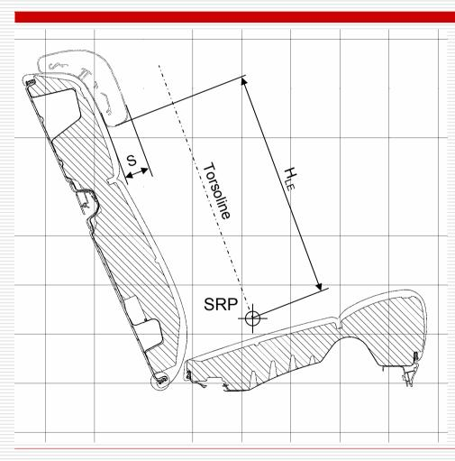
Definition of lower edge of head restraint in non-use position:
