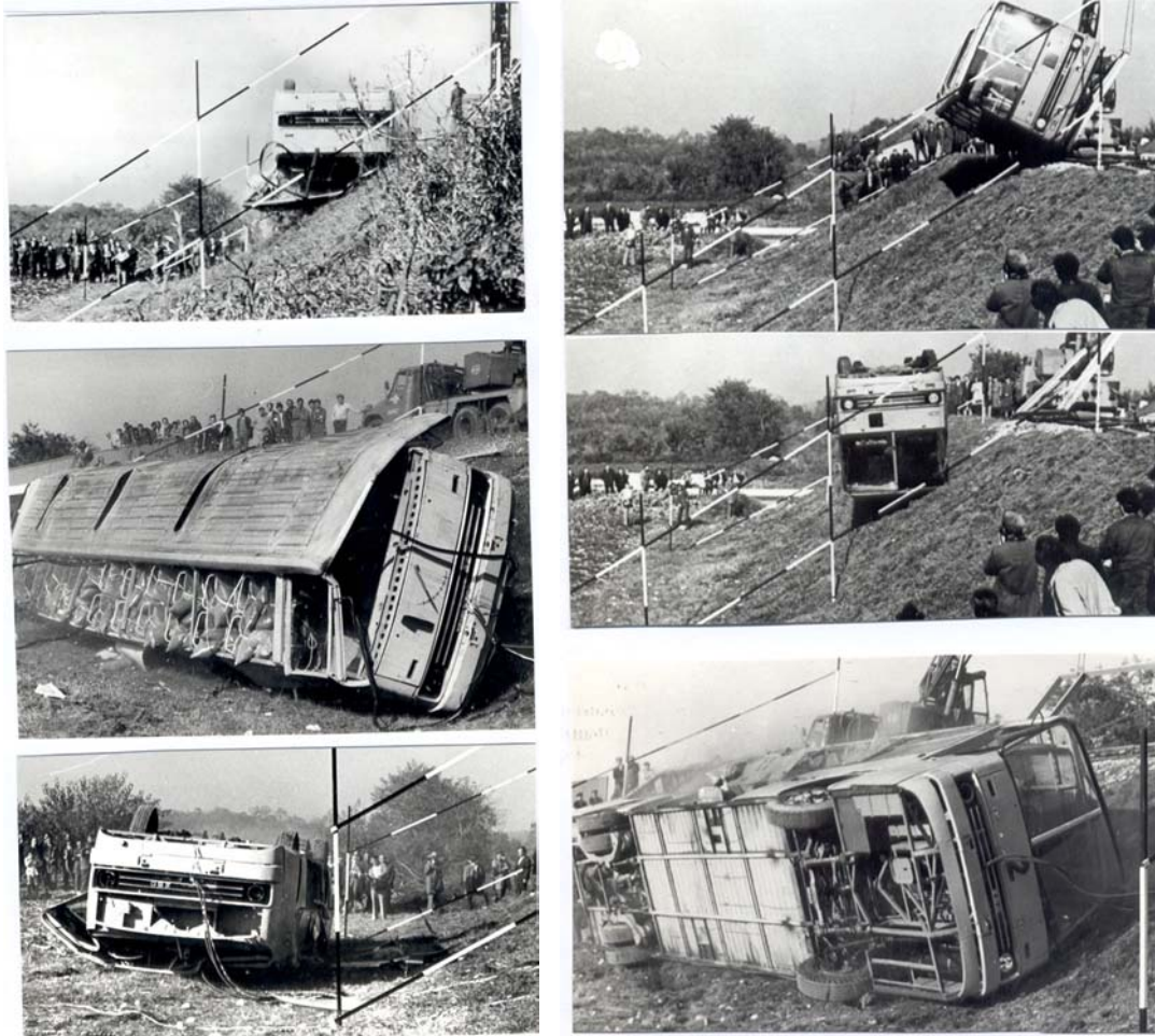
Fig.10. Weak superstructure on steeper slope
