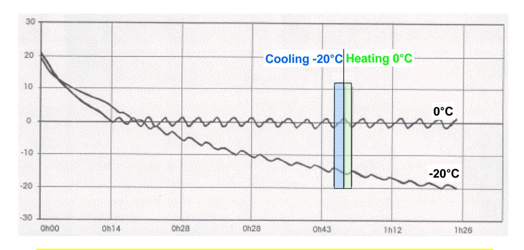
No operation of frozen evaporator at -20°C when the chilled evaporator is cooling at 0°C, therefore reduced runtime of frozen evaporator
