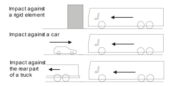
In our opinion, the best way for increasing the driver and passengers bus safety is increasing the distance between driver and front bumper, and using this new distance for the dissipation of impact energy.
