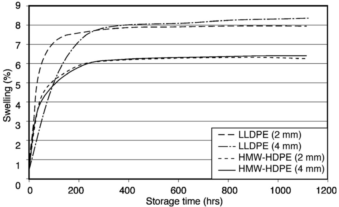
Fig 4 Swelling of HMW-HDPE and LLDPE material as a function of storage time for 2 thicknesses in xylene mixture at 23°C
