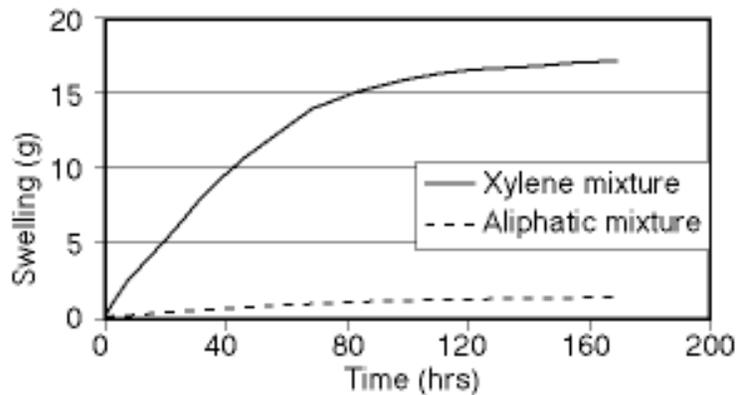
Fig 1 Swelling of 10 litre jerrican after storage with xylene mixture and aliphatic mixture as function of time at 23°C
