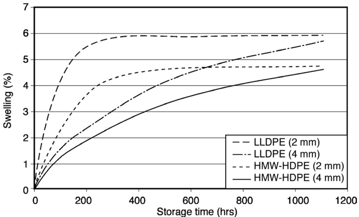
Fig 7 Swelling of HMW-HDPE and LLDPE material as a function of storage time for 2 thicknesses in aliphatic mixture at 40°C
