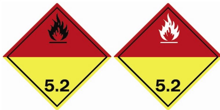
(No. 5.2) Division 5.2 Organic Peroxides Symbol (flame): black or white Background: upper half red, lower half yellow Figure ‘5.2’ in the bottom corner
