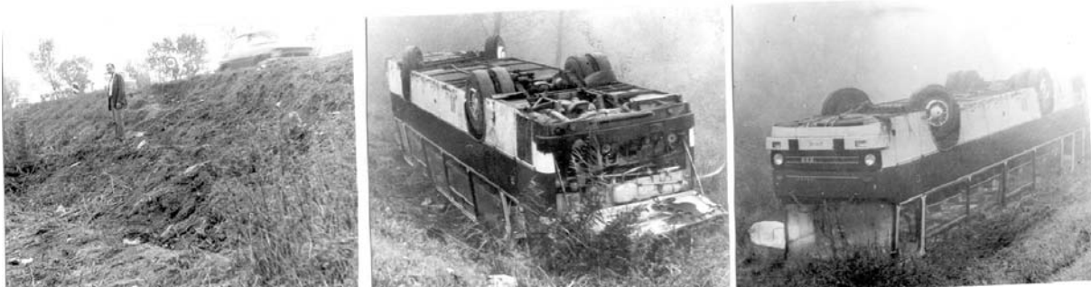
Fig.4. Rollover accident with reinforced superstructure
