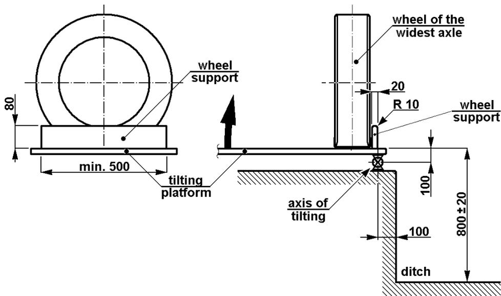
Figure A5.1 - Geometry of the tilting bench
