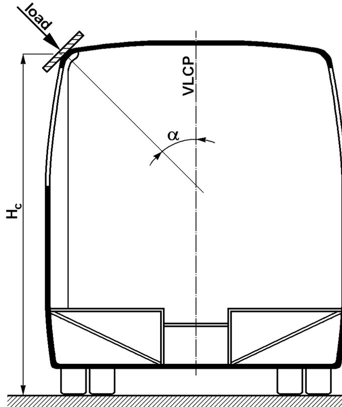
Figure A8. 2 - Load application to the superstructure
