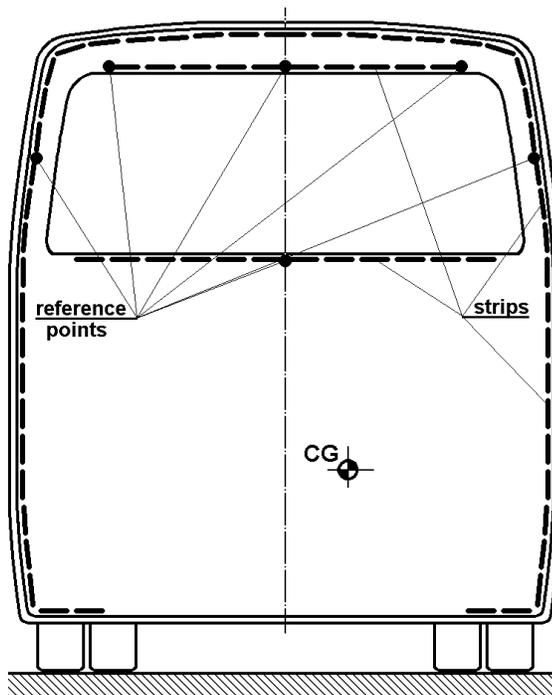
Figure A5.2b - Recommended marking of the centre of gravity position and the contour of the vehicle
