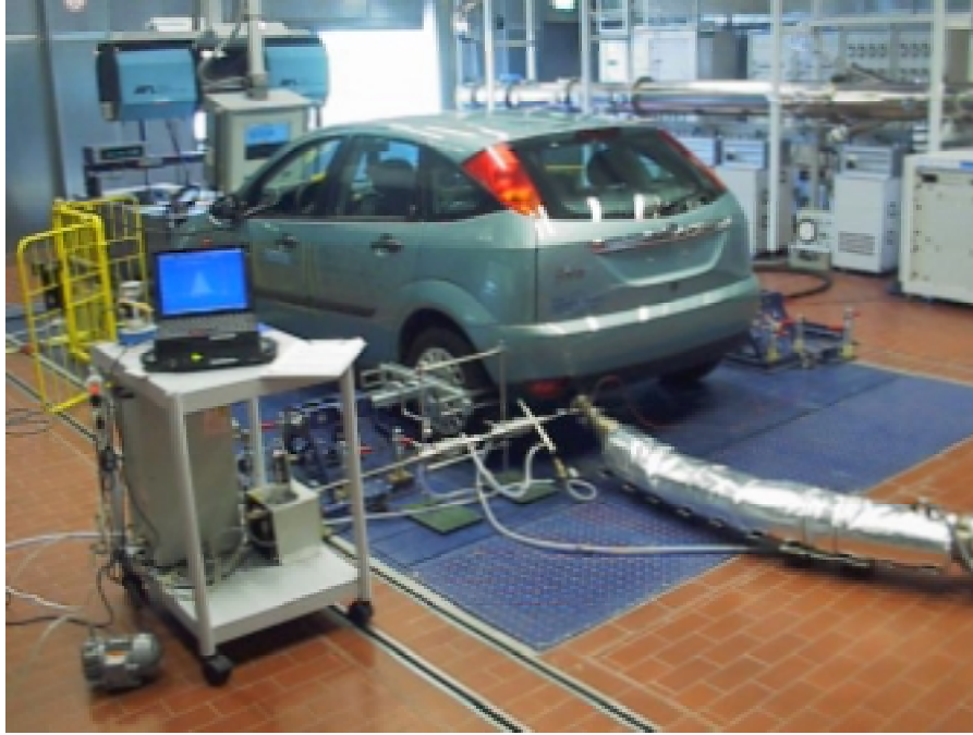
Fig. 1: Dynanometer exhaust dilution & sampling. For direct tailpipe sampling two ejector-pump diluters or a rotating disk diluter (Matter Engineering AG) were used.
