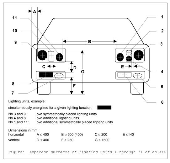
6.20.4.1.2. Additional lighting units, if any, on either side of the vehicle shall be positioned at a distance not exceeding 440 200 mm
