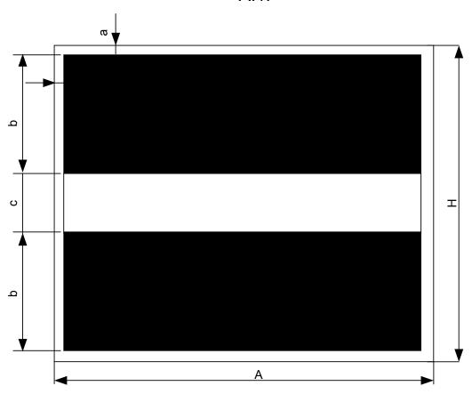
Measurements in mm, in relations to the width of the fairway
