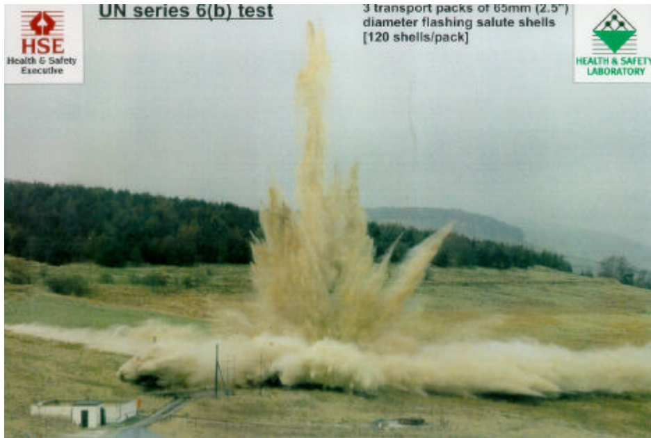
Photo 1 – 6(b) test of 65mm flashing salute shells
