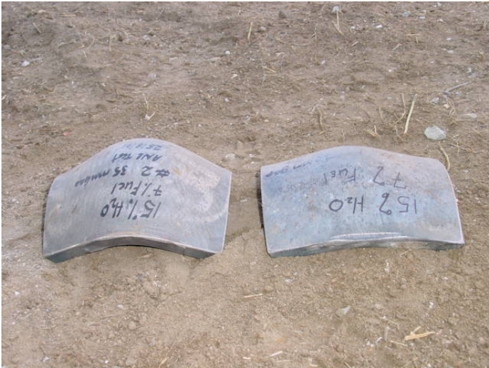
Figure 2 Result of impact on witness plates for SMX ANE1. The 35mm gaps' witness plate is on the left.
