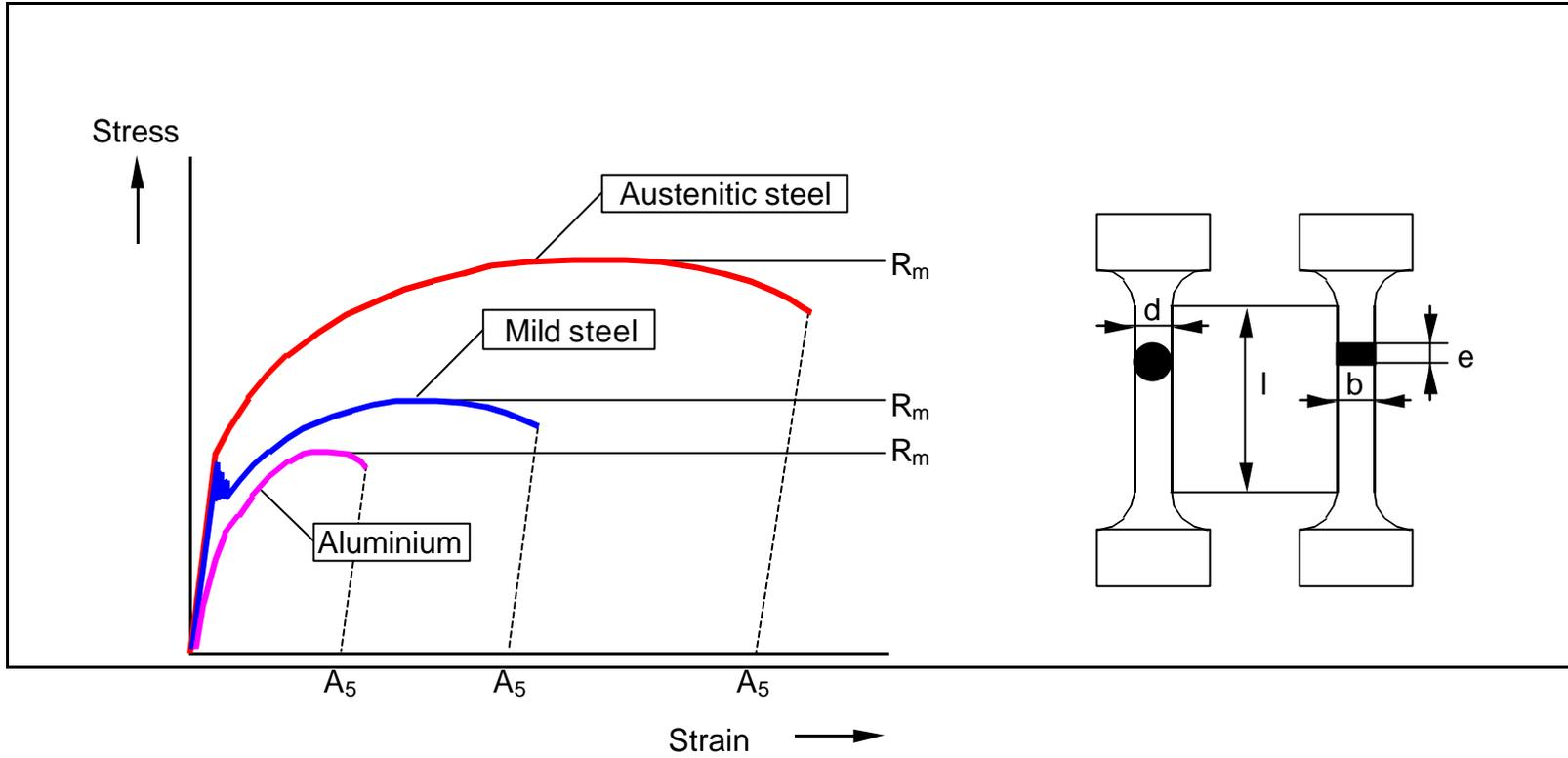
Figure 1: Stress - Strain diagram of typical tank materials
