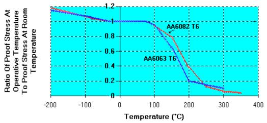
operating conditions at low temperatures. The most widely used distribution equipment for refrigerated liquids operate in the regions of -180°C to -196°C which utilises much of these increased mechanical properties. Although these properties should not necessarily be considered in any pressure calculations, this unique improvement in proof stress is of significant contribution to impact loading on the vessel.
