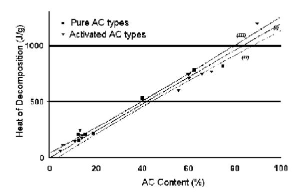
Figure 1: Graph showing the correlation between the energy of decomposition and AC content
