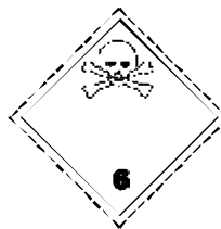
(No. 6.1) Symbol (skull and crossbones): black; Background: white; Figure '6' in bottom corner
