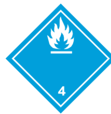
(No. 4.3) Division 4.3 Substances which, in contact with water, emit flammable gases Symbol (flame): black or white; Background: blue; Figure '4' in bottom corner
