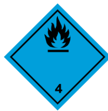
(No. 4.3) Division 4.3 Substances which, in contact with water, emit flammable gases Symbol (flame): black or white; Background: blue; Figure '4' in bottom corner
