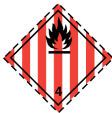
(No. 4.1) Division 4.1 Flammable solids Symbol (flame): black; Background: white with seven vertical red stripes; Figure '4' in bottom corner
