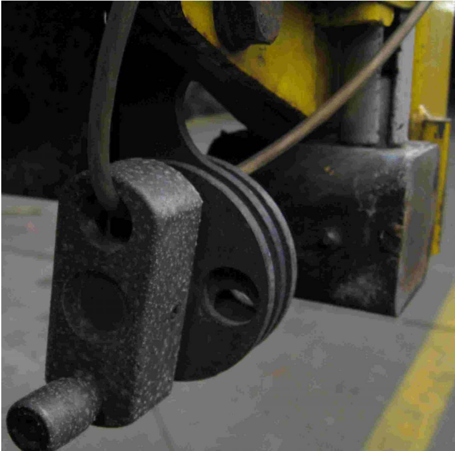
Detail of tensioning device on a TIR vehicle
