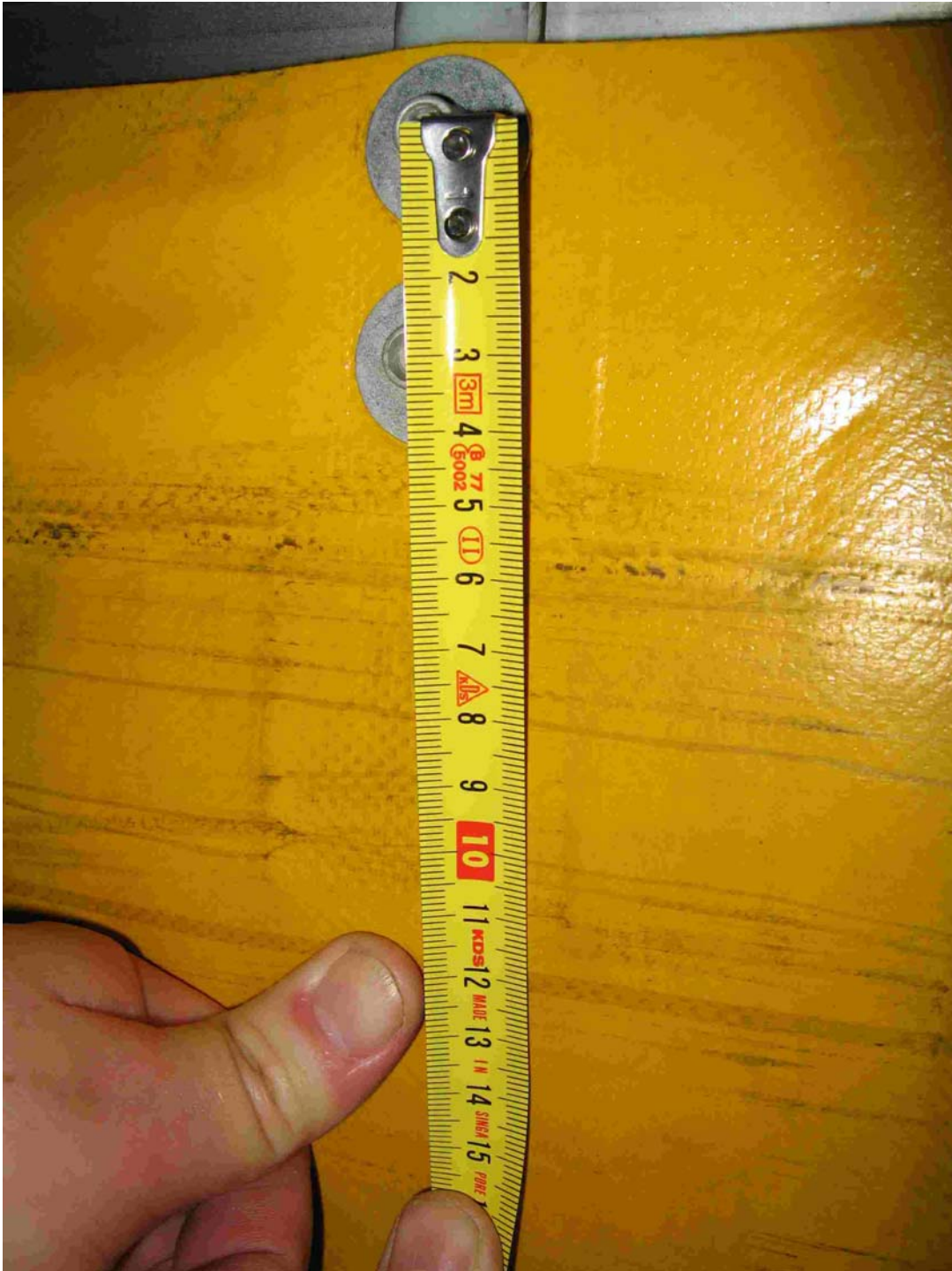
Sheet overlap at the top of the TIR Vehicle
