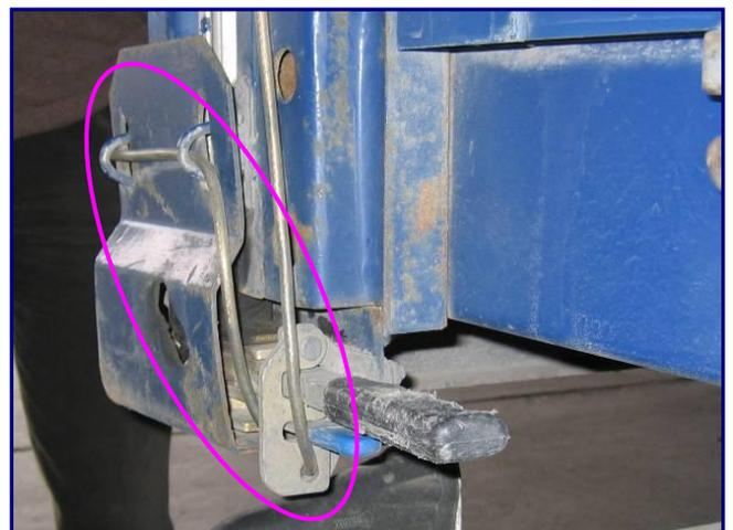
**LEFT:** Ratchet release system – note the height of the square axle: 20 mm only!
