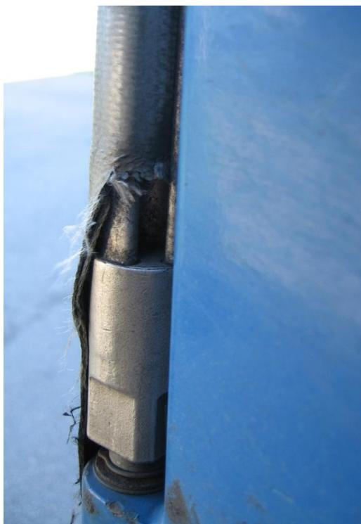
Picture of an end-piece with square lower part. This end-piece (and draw-bar) can easily be rotated by using a normal wrench. Also the opening where the sheet is inserted in the draw-bar is accessible. Note the gap between the sheet and the end-piece (app 2,5 cm) – the sheet can slide this distance inside the draw-bar.
