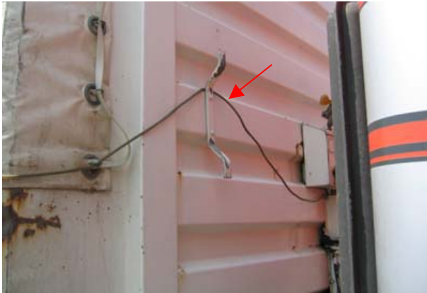
A: TIR-wire hooked up next to the junction box.
