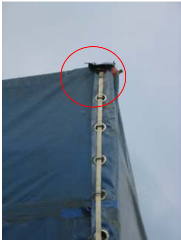
A: Thong - joined outside (with rivets).
