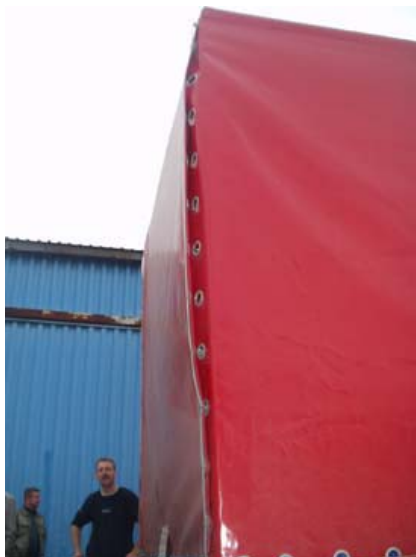
A: Thong not passing through 7 TIR-rings.
