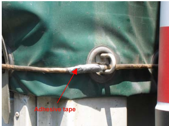
A: TIR-wire wrapped with adhesive tape. (Camouflage)
