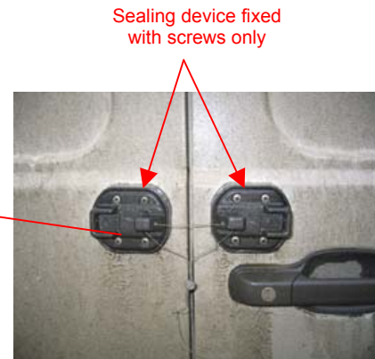
D: Only 4 screws need to be removed - and the device is ineffective.
