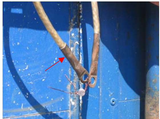
B: End-pieces made of copper pipe – just pressed onto the rope. Easy to open and put back on.
