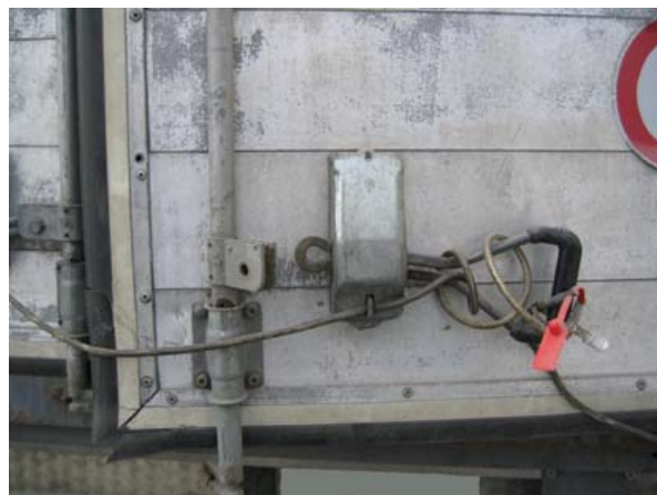
D: Handle disconnected, locking rod turned - and the door is open! - And it is just as easy to put back again!
