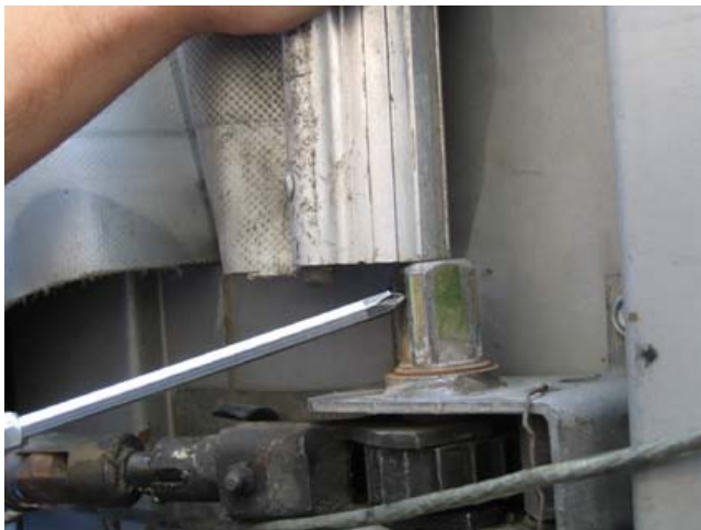
C: When released, it is easy to lift the tensioning bar off the base and get access to the load.
