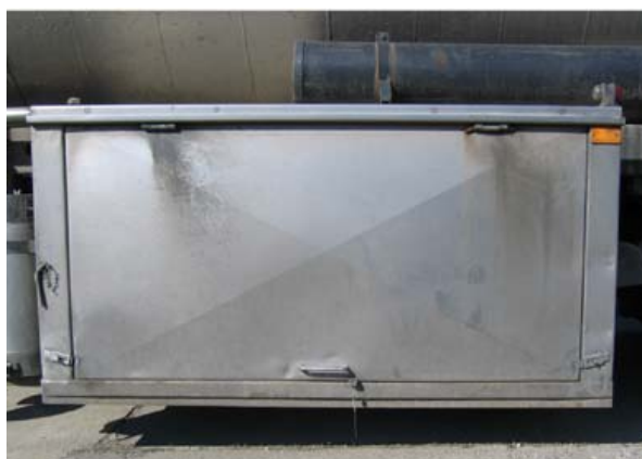
B: Hatch for the compartment - handle, locks and the customs seal.
