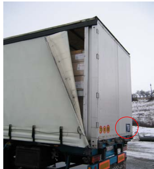
D: Limited - but unacceptable access to the load. Note the TIR approval.
