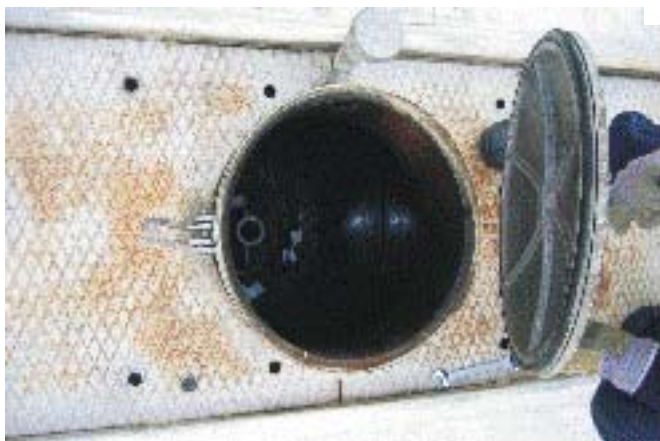
C: Center bolt removed - handle released from the main axle.
