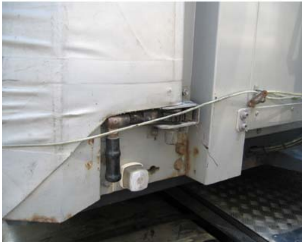
A: Trailer equipped with tensioning device - type "catch and pawl".
