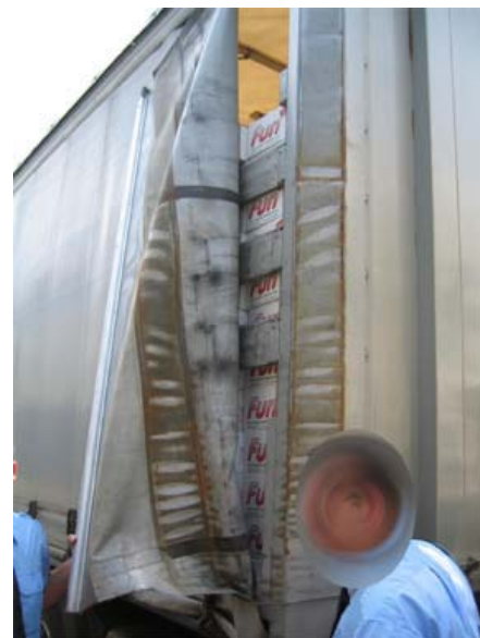
D: Limited - but still unacceptable - access to the load.
