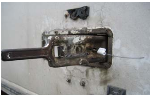
E: Semi-lock seal stays outside the handle. Now it is possible to pull the handle and open the door.
