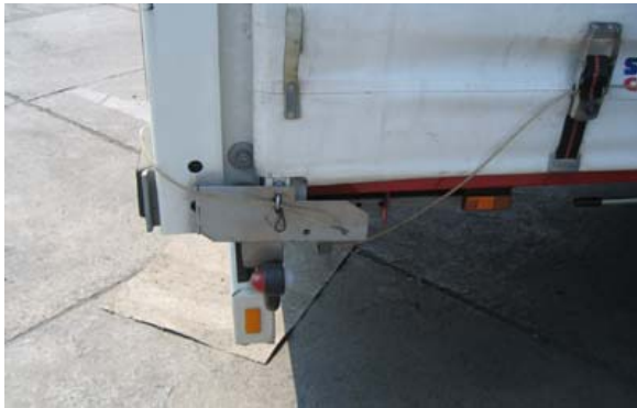
B: Security measure: A metal plate - blocking the handle for the tensioning device (type "worm drive").
