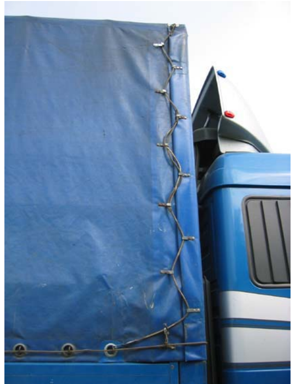
B: No thong - only elastic rope and hooks. (Front view of the truck)
