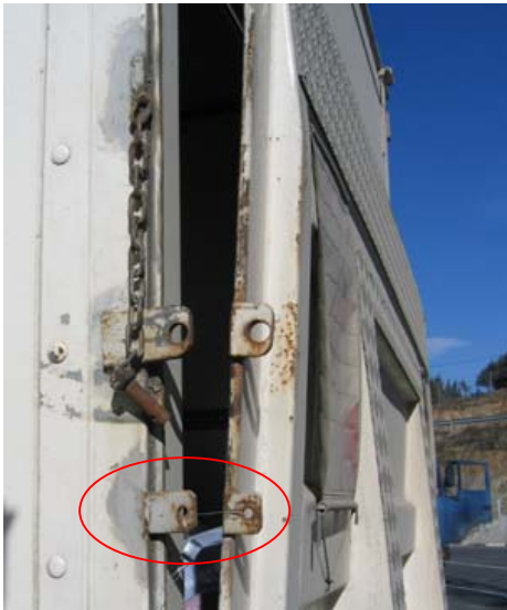
D: Hydraulic system activated – the ramp opened as much as possible without breaking the seal.
