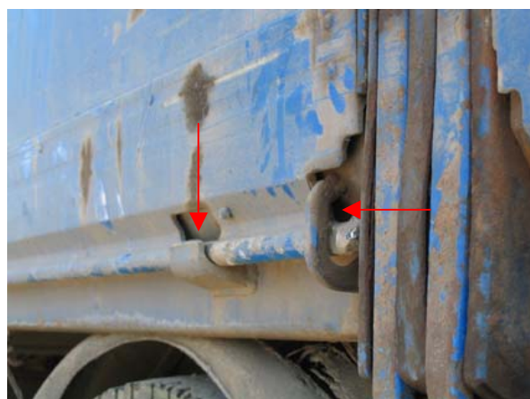
C: Note the “open” hinge and the spacious ring.
