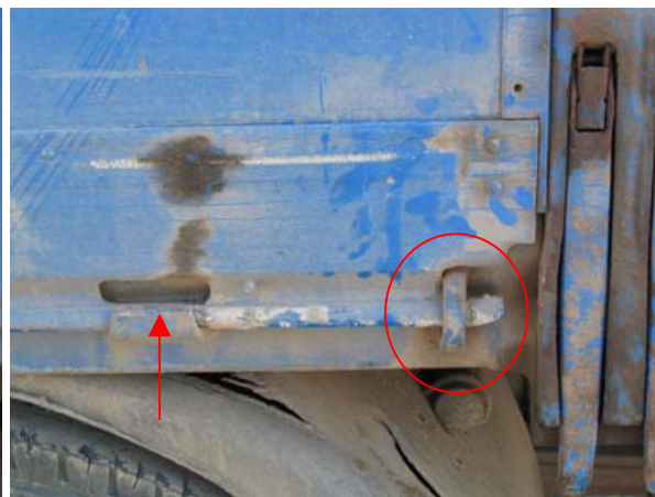
B: The “open” hinge, the solid metal ring and the vertical maneuver handle for the lock system.
