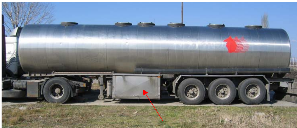
A: Tanker equipped with a special compartment for pipelines and valves.
