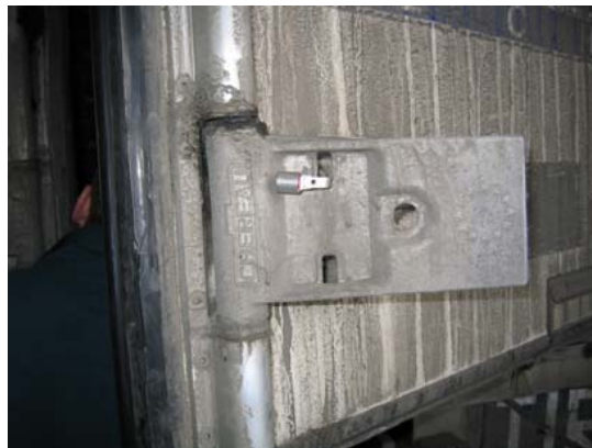
D: Handle turned, locking rod activated - door open - seal remain unbroken.
