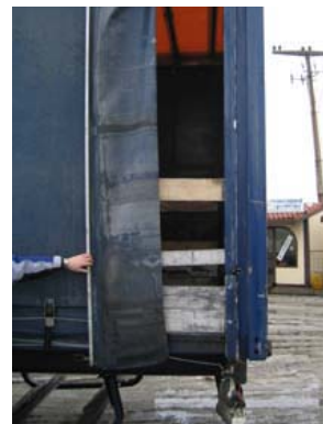
F: Tension bar released - access to the load.
