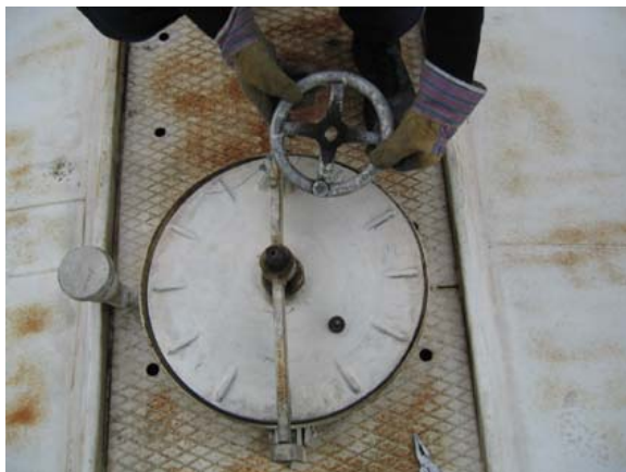
C: Center bolt removed - handle released from the main axle.
