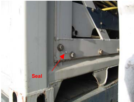
A: Lower part of the frame, bolts and seal for the refrigerator unit.
