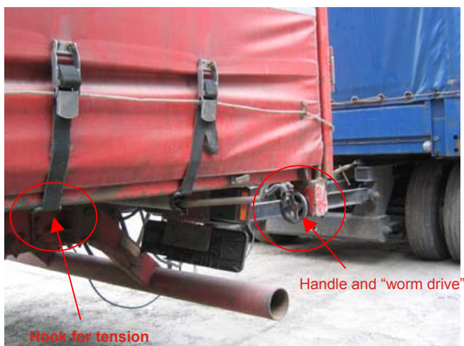
A: Handle not secured - TIR-wire not passed through the handle.
