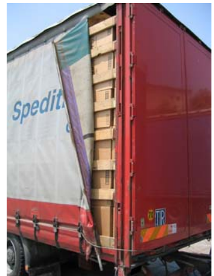
B: System released - tensioning bar lifted off the base - sheet opened 50 cm.
