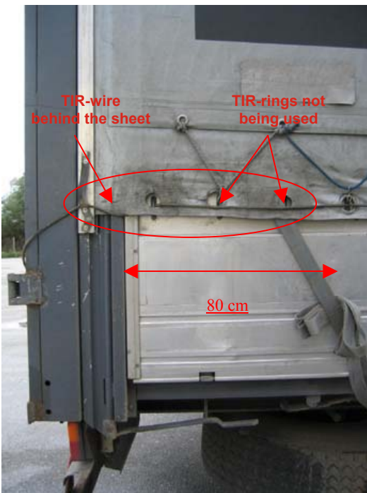
B: TIR-wire wrongly passed and TIR-rings not being used.
