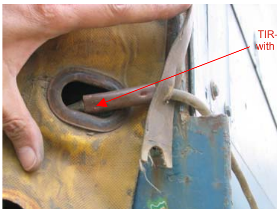
A: TIR-wire cut or broken - repaired with a piece of copper pipe.
