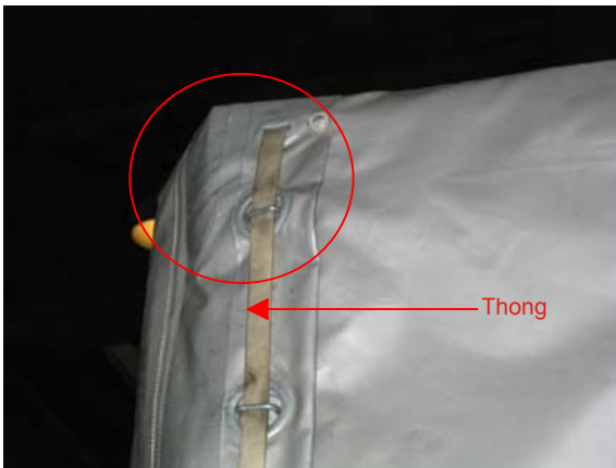
A: Thong - inserted through a special hole for passing through all layers of the sheet. (Upper front part of the trailer)
