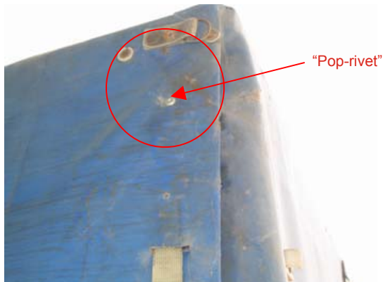
A: Thong fitted with a “pop-riquet”. Note that is a brand new rivet! OUTSIDE view.
