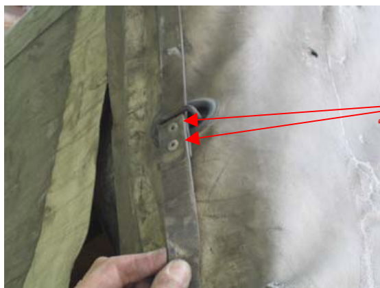
D: Thong, cut or broken, repaired - joined with blind rivets.
