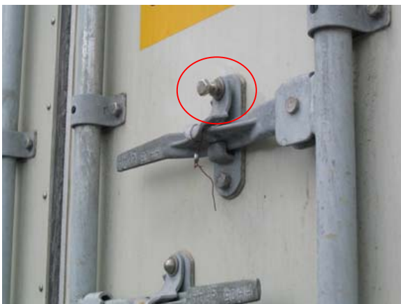
C: Bolt almost removed.
