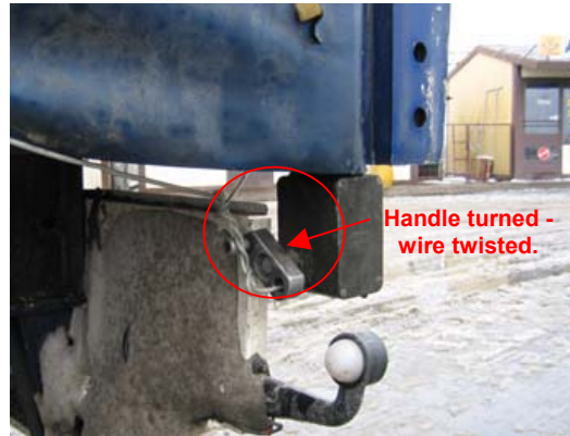
D: But this long wire will just get twisted when the handle is turned and the tension bar can be lifted off the base.
