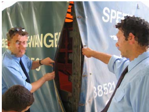
D: Good access when thong is removed.
