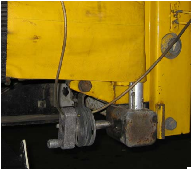
Tensioning device mounted on the TIR vehicle - providing efficient security.
