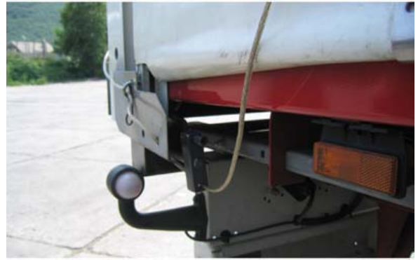
C: Security measure: The metal plate - secured by the TIR-wire blocking the handle for the tensioning device (type "worm drive").
