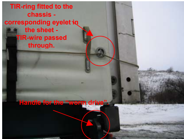
A: Security measure - TIR-ring and corresponding eyelet in the sheet.
