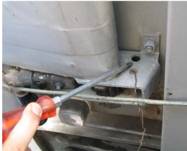
B: The TIR-wire not passed through the specified holes for blocking the pawl.
