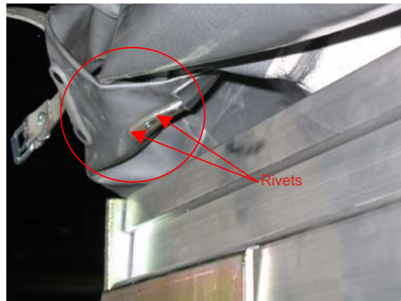
B: Thong secured - mounted to the INNER layer of the sheet. (Upper front part of the trailer)
