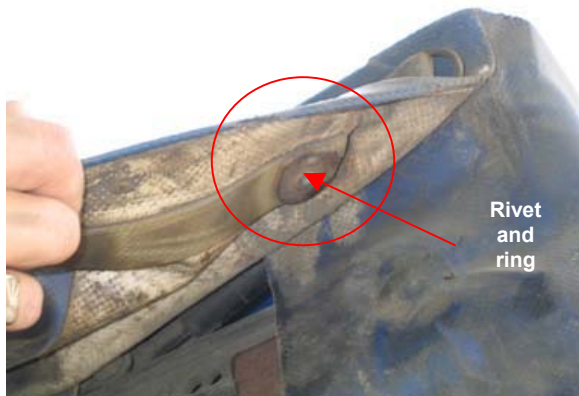
C: Thong fitted only to the outer layer of the sheet - making it easy to replace the rivet.
