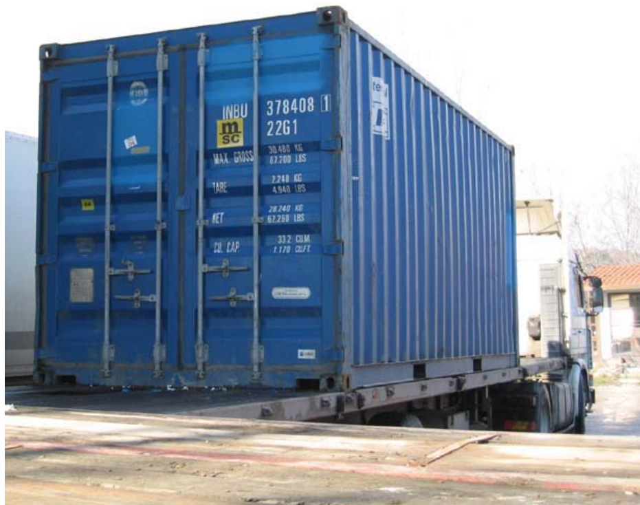
A: Standard 20' container placed on a trailer. Container only having doors.
