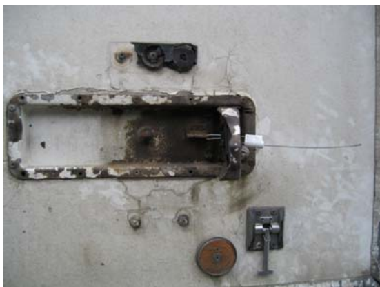
C: The wire can pass the sealing device and the handle can be released as much as 75E.
