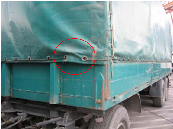
A: TIR-wire hidden behind the sheet.
