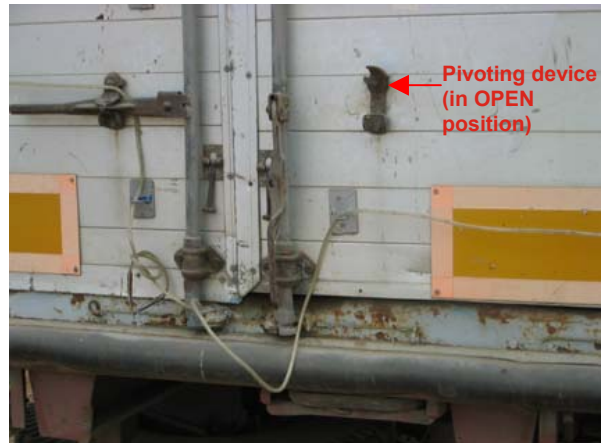
B: Pivoting device OPEN, handle and locking rod released.
