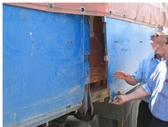
D: Release the lock system, lift the sideboard off the hinges, and there is access to the load compartment.
