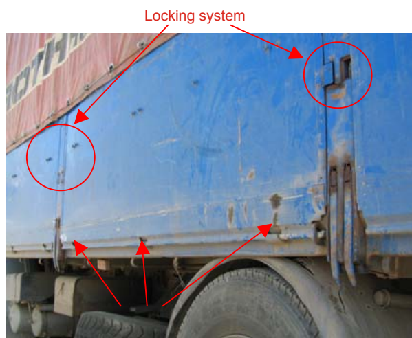
A: Open hinges - the sideboard only being secured with the locking system and a single metal ring.
