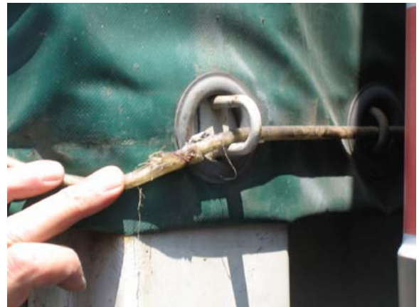
B: Removal of the tape revealed the jointed TIR-wire.
