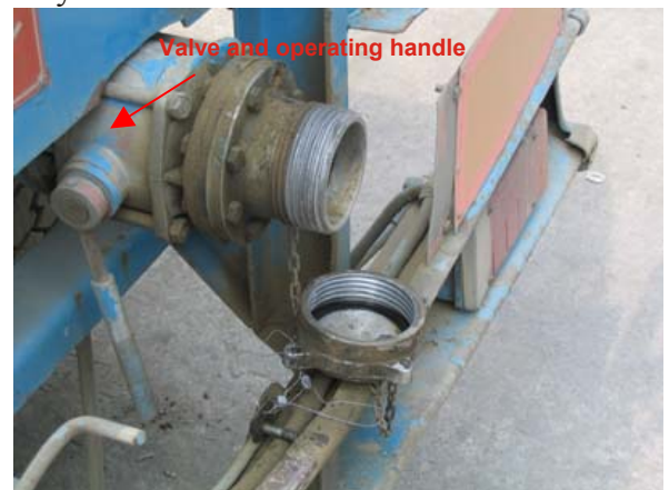
D: End cover removed - now it is possible to discharge - just activate the valve.
