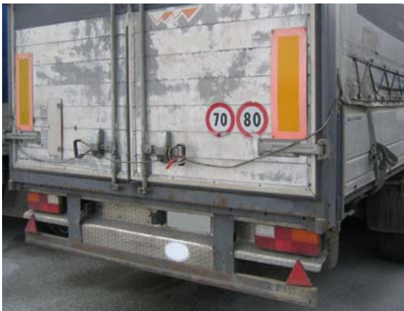
A: Standard conditions fulfilled – apparently acceptable security and sealing.
