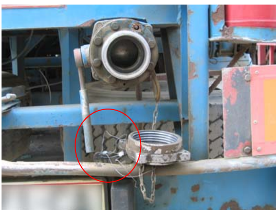
C: Bolt and plate dismantled - now only attached to the end cover by the strings and seals.
