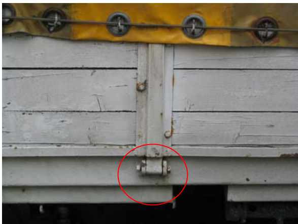
A: Unsecure hinge for sideboard. (Truck of an earlier date.)
