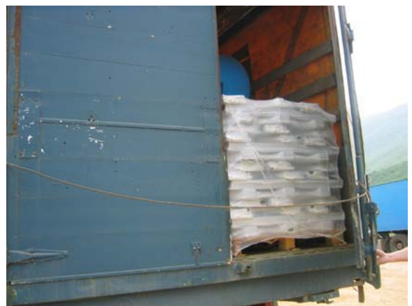
D: Just 1 meter of extra wire makes it possible to open the door widely.
