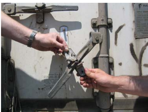
D: Back plate and pivoting device removed.
