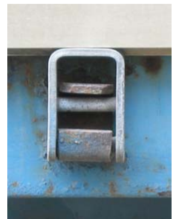
C: “Self-securing” hinge - sideboard. (Old-fashion version)
