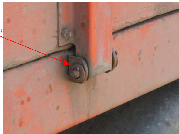
B: The unsecure hinge can be adapted by cutting off the head and nut leveling the outer of the bearing and then welding.
