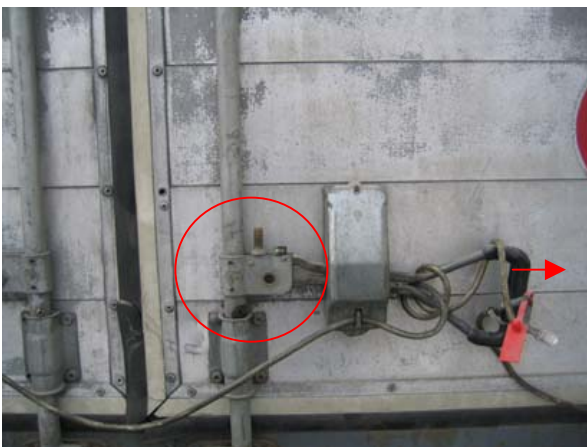
C: Center-bolt removed - handle slightly pulled.
