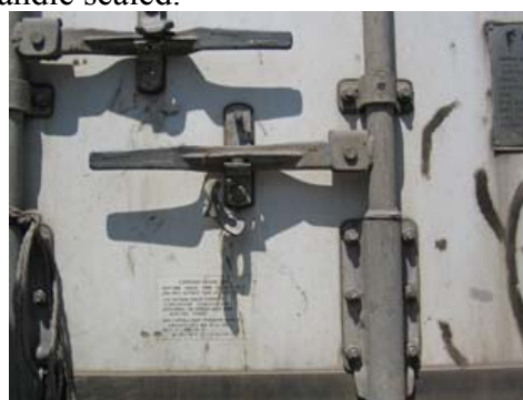
C: Upper nut removed - pivoting device still attached to the handle and back plate.
