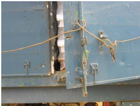
C: TIR-wire too long - maneuver handle not secured. Wire not even passing through the hole in the pivoting device and handle.
