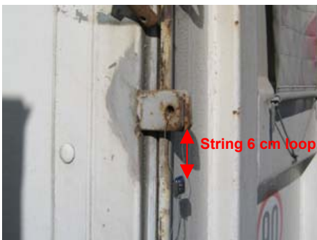
B: Seal and sealing device. Note the long string - leaving a loop of approximately 6 cm.
