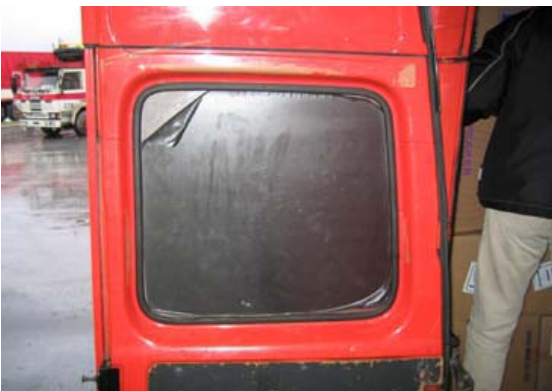
D: Rear door - window not secured – only adhesive plastic foil to diminish visibility.
