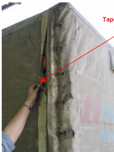
C: The sheet repaired with adhesive tape only. Unauthorised (homemade).
