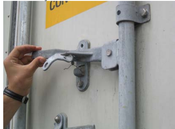
D: Pivoting section and customs seal still attached to the handle.
