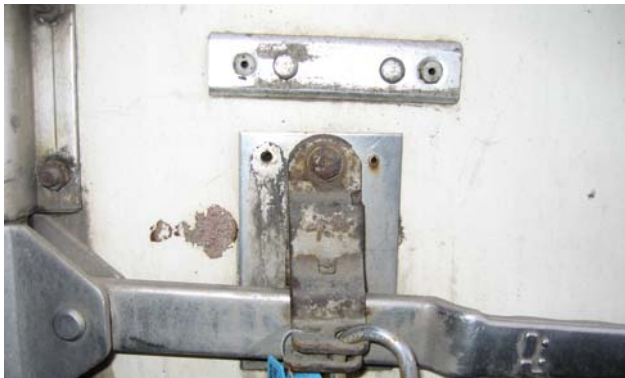
B: Pivoting Customs sealing device appear to be assembled from parts made of different metals – iron and stainless steel. Normally all parts for such devices are made of stainless steel.
