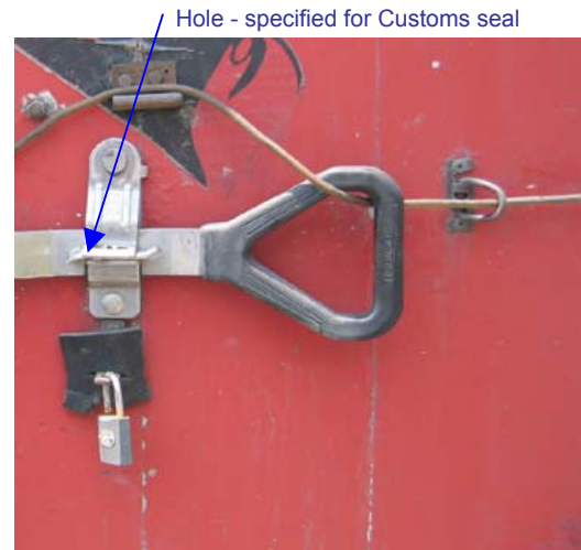
B: Pivoting device - specific hole for affixing Customs seal. Handle NOT secured.
