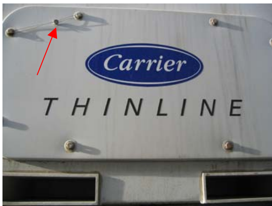
C: Two examples of sealed hatches - a part of the refrigerator unit.
