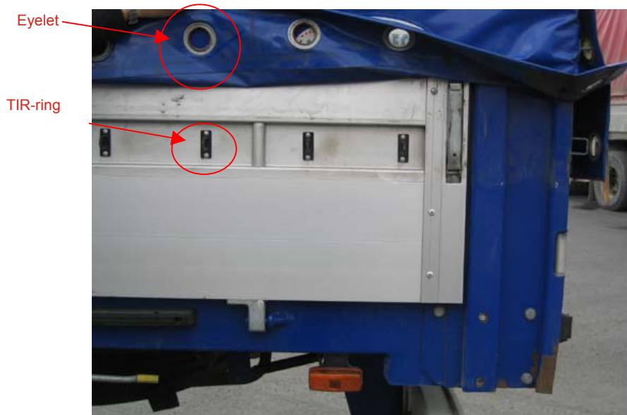
A: Properly mounted TIR-rings and eyelets.
