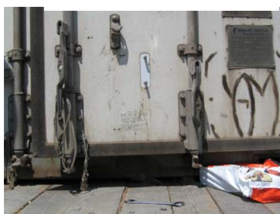
E: Locking rods released - door slightly opened.
