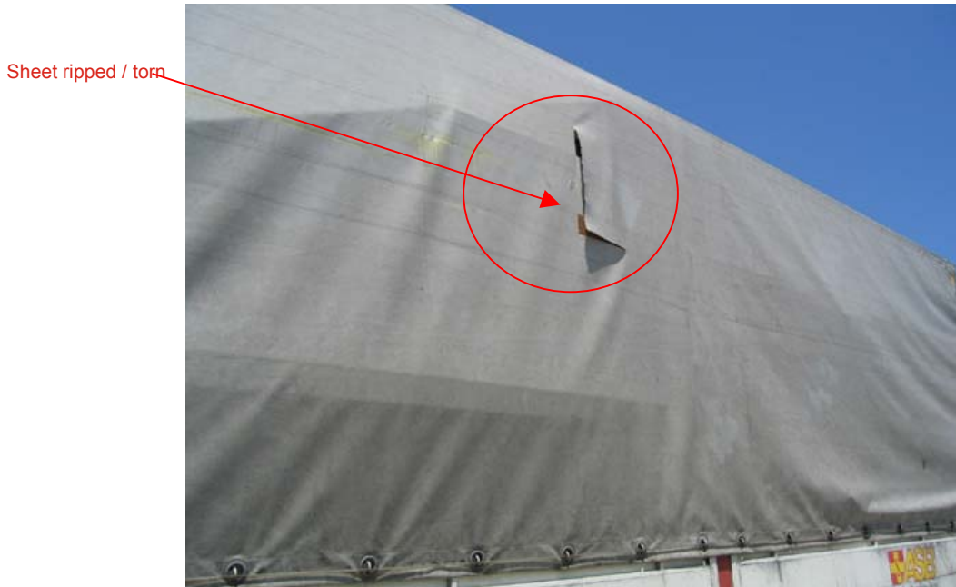
A: Sheet ripped during journey, with rather extensive damage. This trailer should NOT be allowed to continue to transport under customs seal - unless it is repaired.
