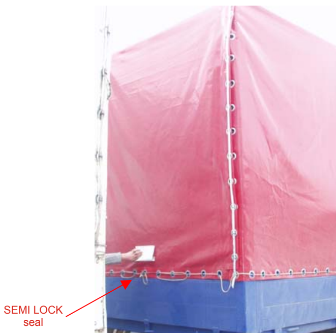
A: Thong not passing through 7 TIR-rings.
