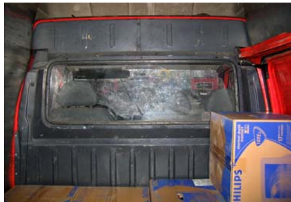
C: Window between the cabin and the load compartment - window not secured.
