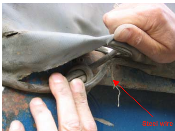
C: Broken TIR wire repaired - two loops made, the ends being secured by thin steel wire, twisted.
