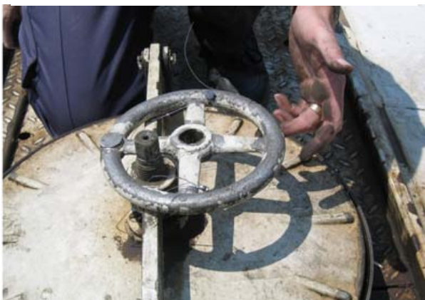
D: Handle removed from the main axle.
