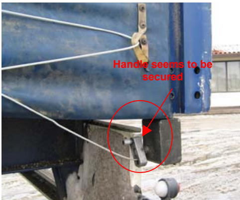
C: Handle seems to be secured - wire passing through.
