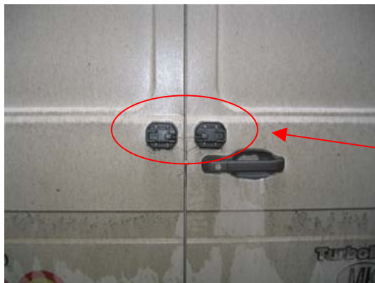
C: Sealing device - homemade - the two plastic bits fixed with standard screws.
