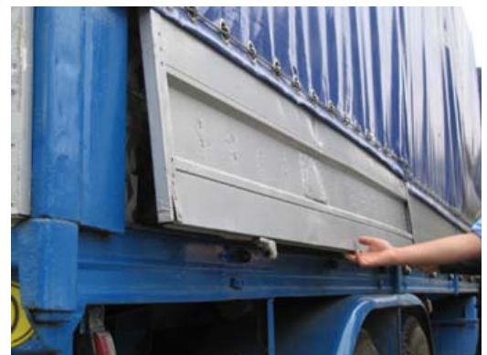
D: Limited - but still unacceptable - access to load compartment.
