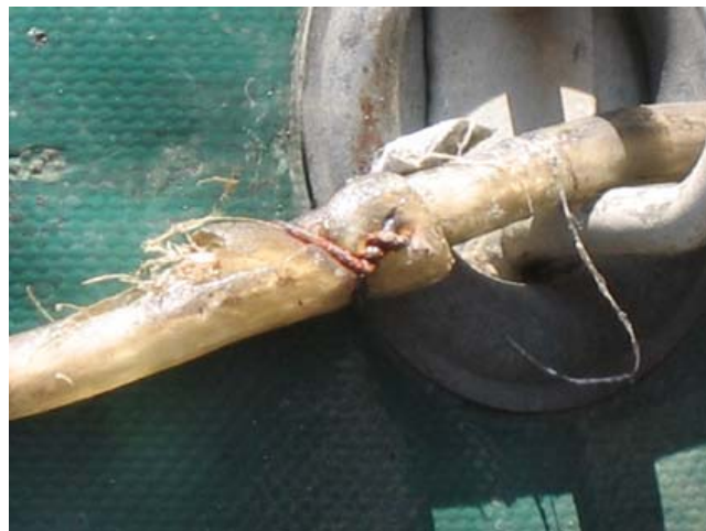
C: TIR-wire jointed with a piece of wire – just twisted and easy to replace.
