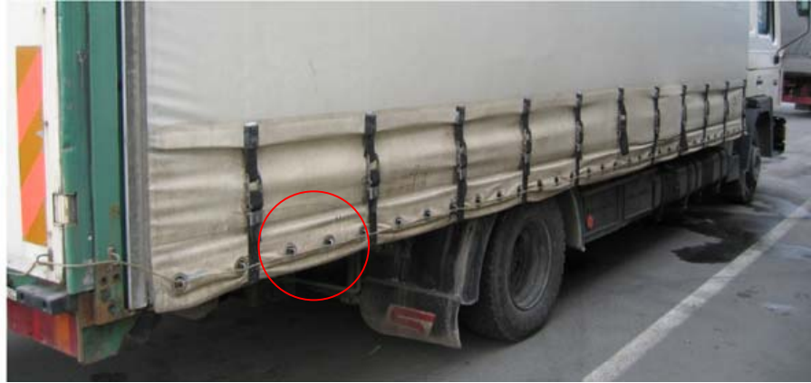
A: Sliding sheet secured by: TIR-rings welded to the chassis, sheet equipped with corresponding eyelets and finally secured by the TIR-wire.
