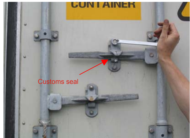
B: Only one bolt has to be removed.
