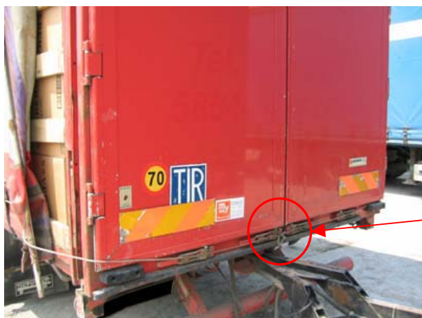
A: Handle not secured - TIR-wire not passed through the handle.
