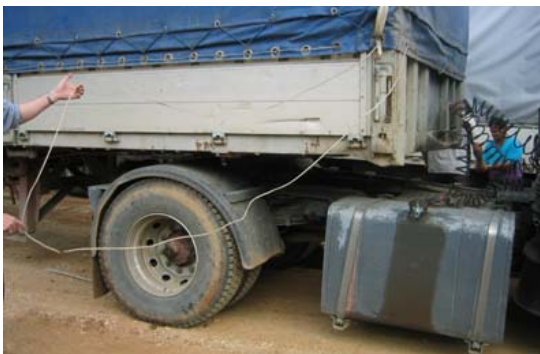
C: TIR-wire, extra length hidden and poorly camouflaged.
