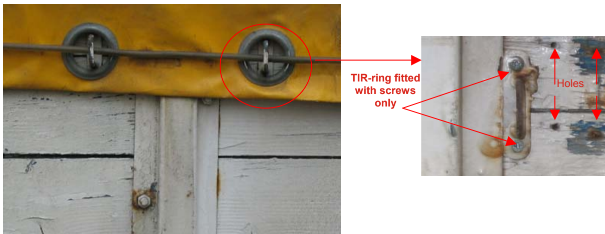
A: Truck with wooden sideboards - it is easily spotted that the TIR-rings have been moved several times. Note the brand new screws.
