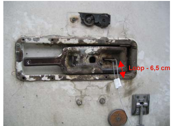
B: Sealing device and "Semi-lock" seal. Note the loop - 6,5 cm!
