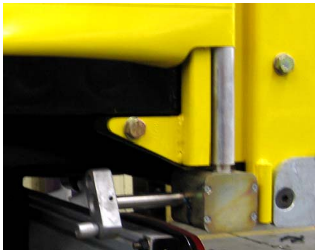
Tensioning device mounted on the STANDARD vehicle. This device provides no security at all!
