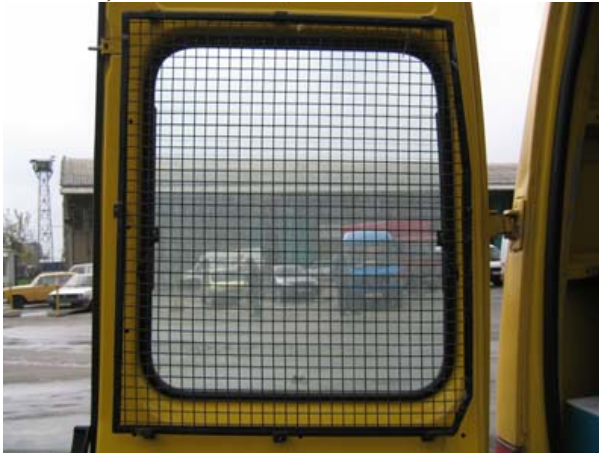
A: Rear door - window secured by metal gauze.
