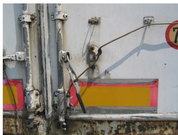
D: Maneuver handle in free position – and the door can be opened.
