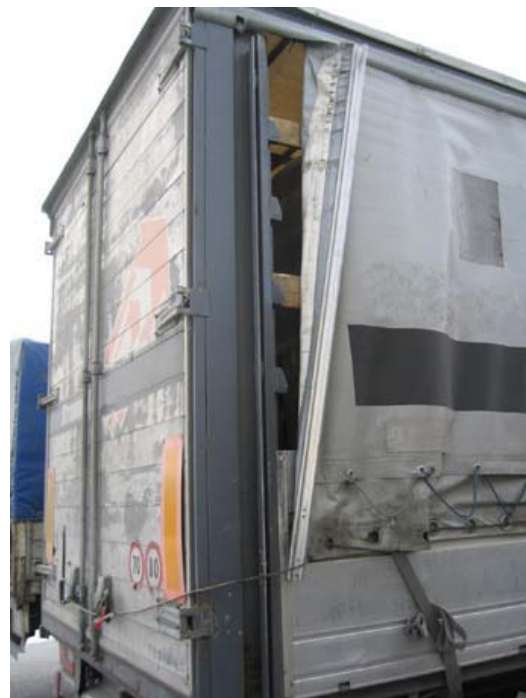
C: Access to the load - it is possible to slide the sheet 80 cm.
