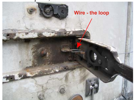
D: Wire can pass - visible behind handle (inside).
