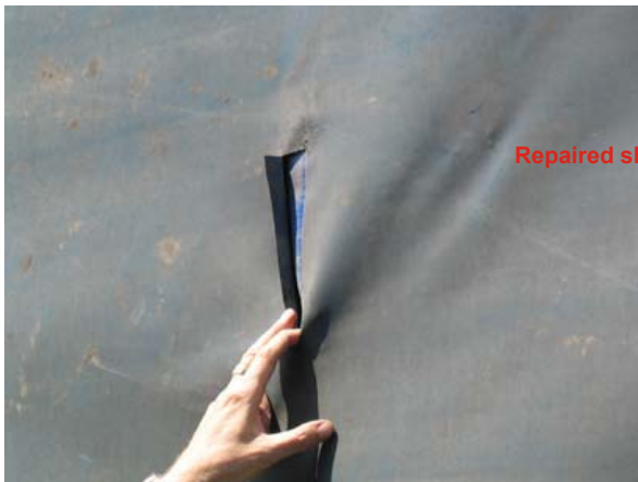
B: Sheet ripped during journey, with minor damage. Dependent on the commodity being transported, this trailer COULD be allowed to complete the current journey - but should NOT be able to carry out further international transport without being repaired.
