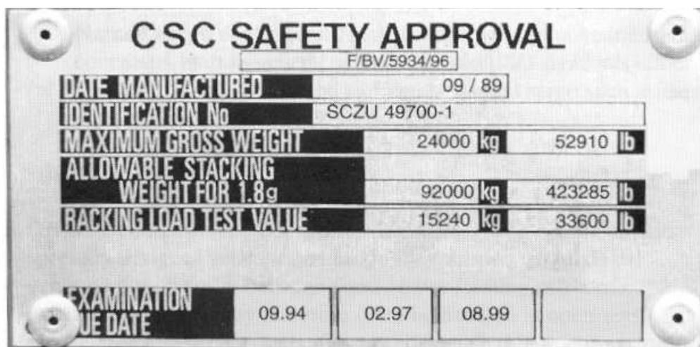
Figure 1: Example of a CSC safety approval plate
