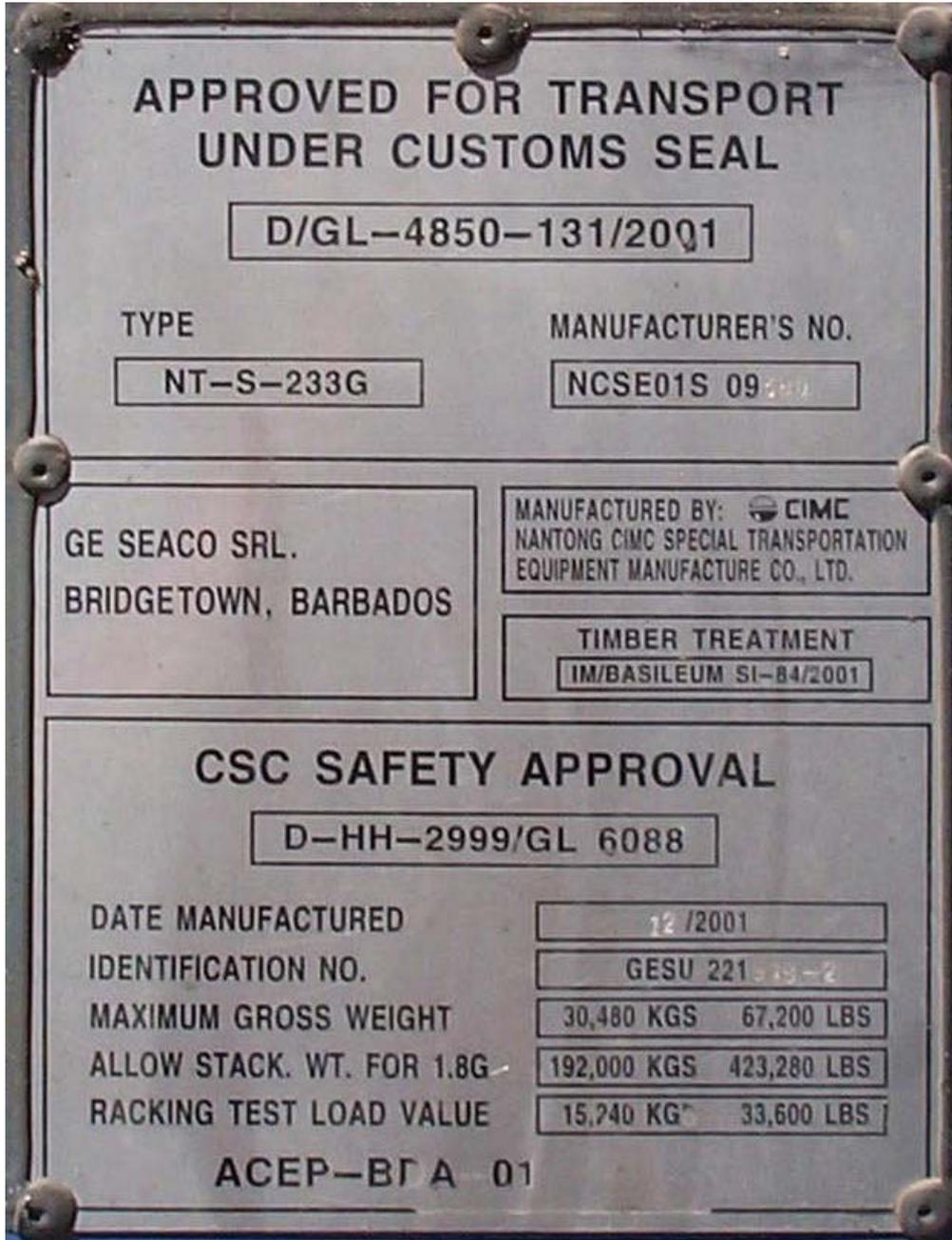
Figure 3: Example of a consolidated approval plate
