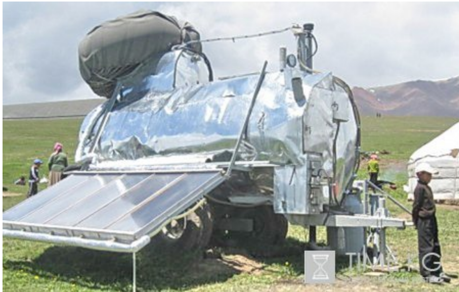
Figure 7 – Portable biogas plant БЭМ-5М
