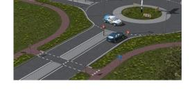
Vehicle arrives at a multilane roundabout with a multi-laned entry and exit by the system based on entered destination or driver instruction. The vehicle has to lane change or cross a lane to exit the roundabout. The roundabout may have lane markings or predefined paths.
