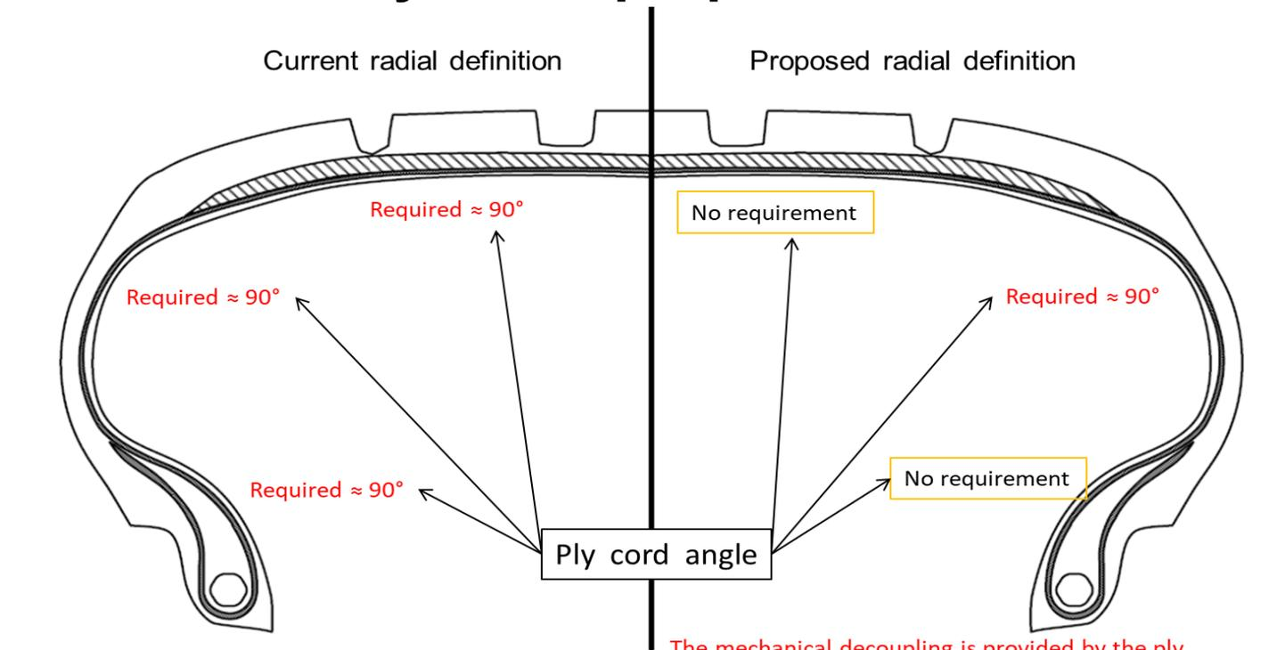
The mechanical decoupling is provided by the ply cords laid at substantially 90° in a zone between the bead and the inextensible circumferential belt.
