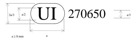
The above Unique Identifier shows that the type concerned has been approved and that the relevant information on that type-approval can be accessed on the UN secure internet database by using 270650 as Unique Identifier. Any leading zeroes in the Unique Identifier may be omitted in the approval marking.
