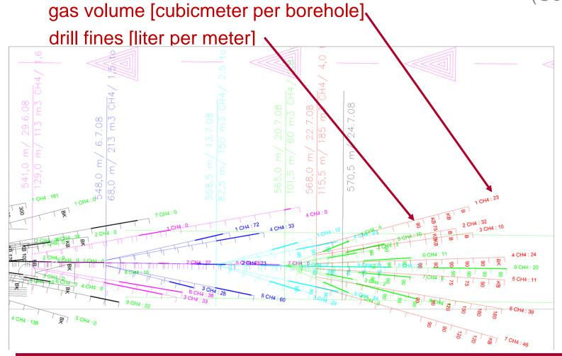
**K**<sub>10</sub> **seam**Methane levels and volume during relaxation drilling (Kazakhstan)
